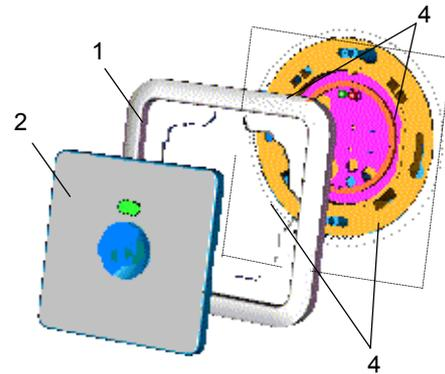
The bases (3) of the cover (2) must engage in the cutouts of the cast component (4).
