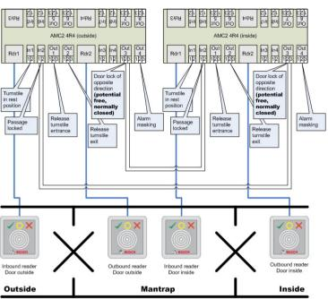
Mantrap configuration with two turnstiles (DM 03a) which are distributed across two controllers.
