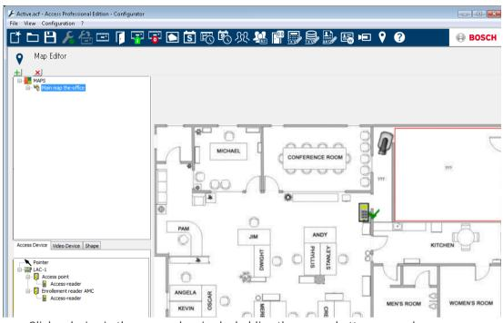
Click a device in the map and resize by holding the mouse button pressed,
