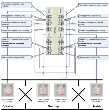
Connections to the door locks for the opposite direction ensure that only one of the turnstiles can be opened at any one time.
