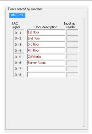
As a standard, one AMC2 can be used for 8 floors. It is possible to increase this number under the following preconditions:
