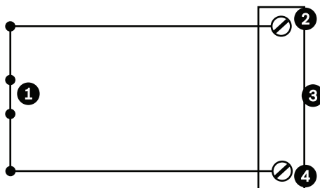
Figure 10.4: N.C. Normally Closed Non-supervised Connections
