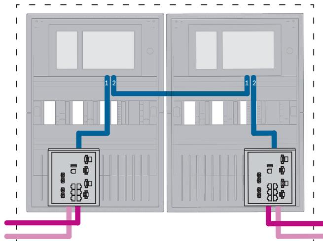
Figure 7.7: Connect Ethernet networks with redundant panels
