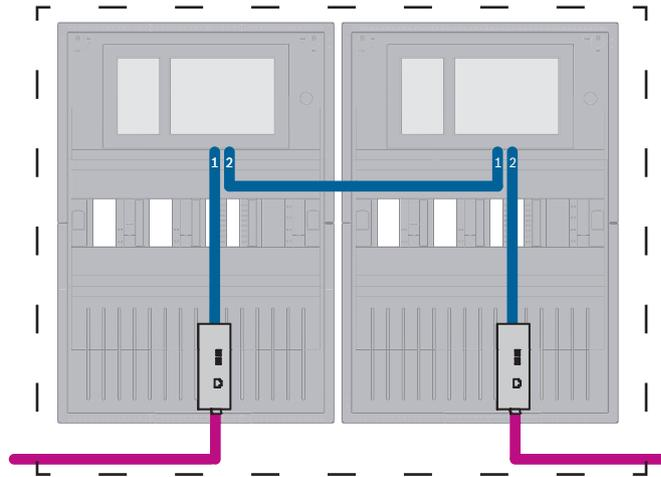
**Figure 7.4:** Panel network over Ethernet with redundant panels
