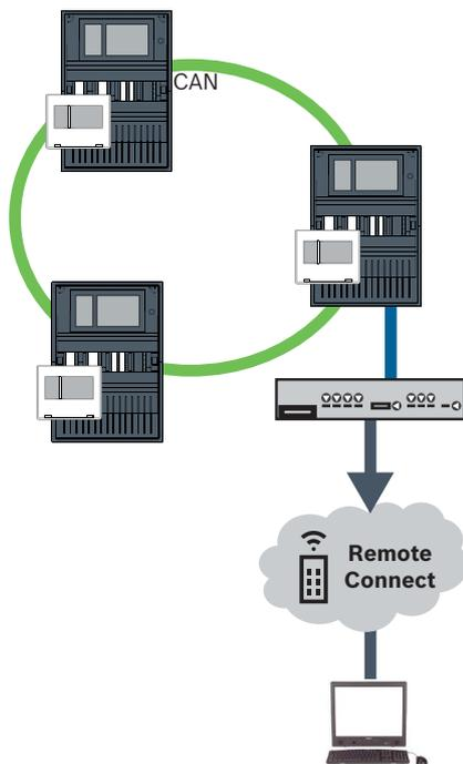
**Figure 8.2:** Remote Connect in a CAN loop
