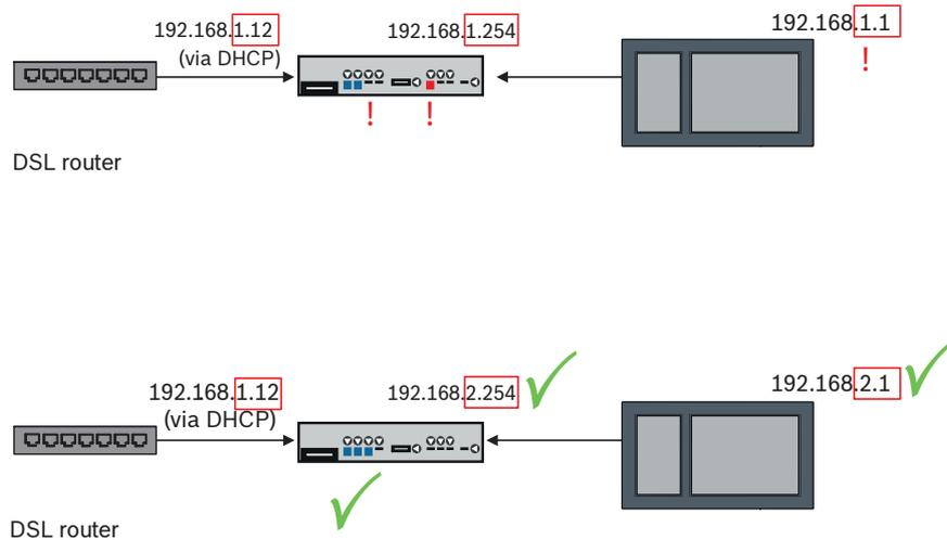
A Secure network gateway detects overlapping sub-networks unambiguously: The Alarm LED is blinking continuously.
