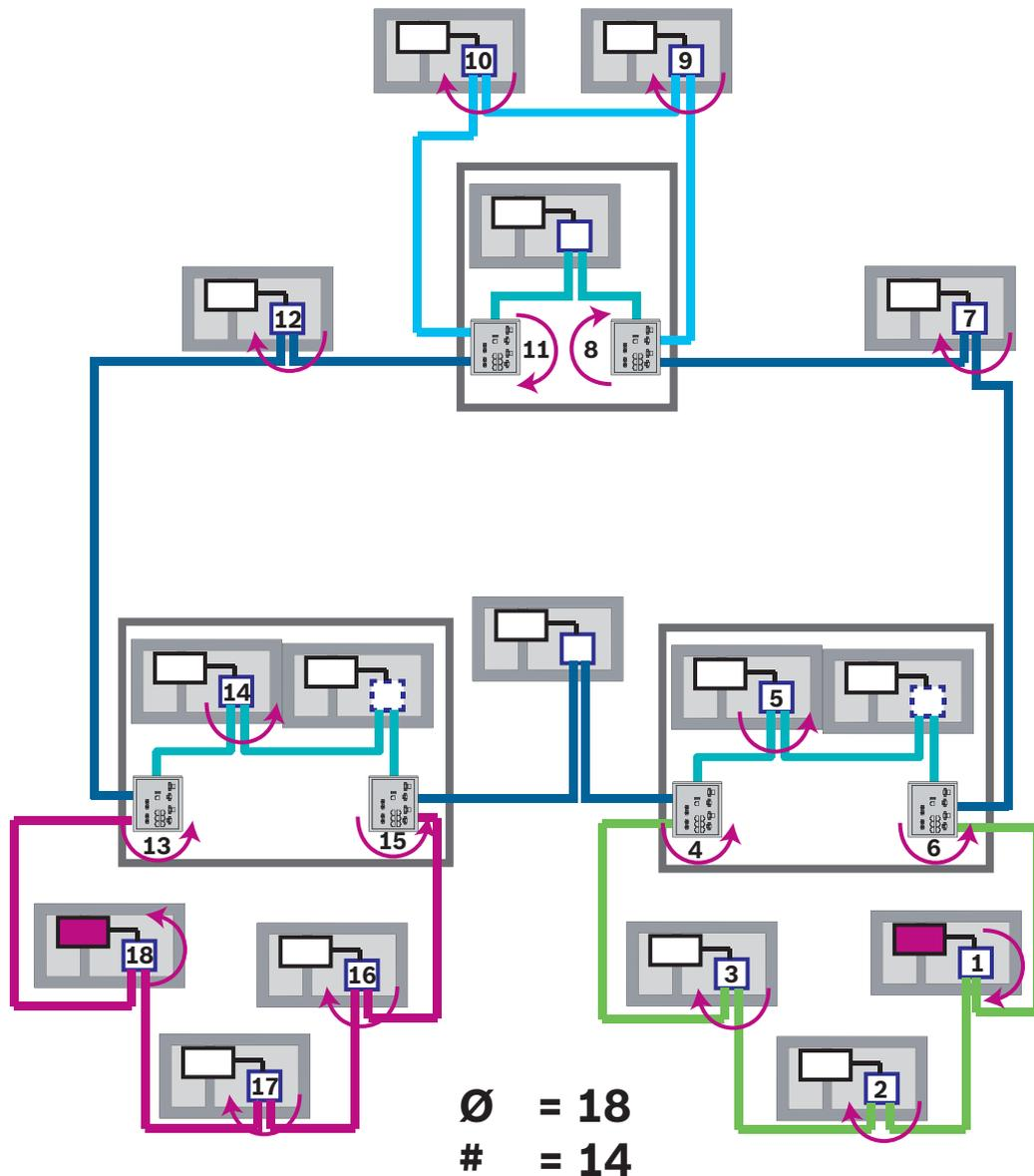
**Figure 5.3:** Network diameter of a backbone with sub-loops
