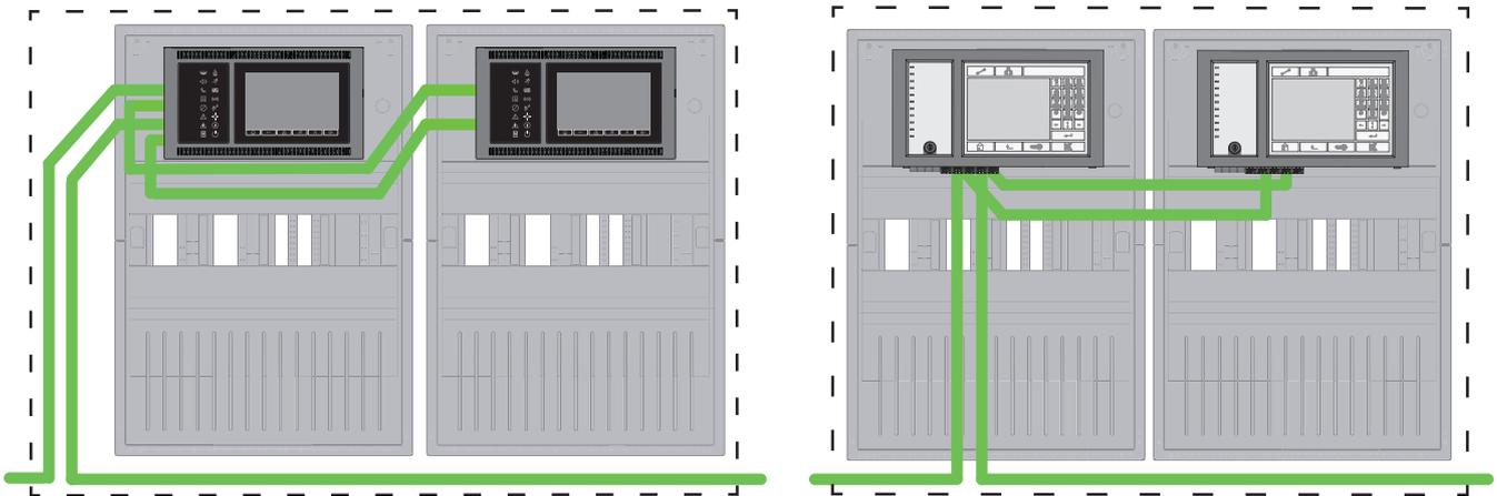
**Figure 7.5:** Panel network over CAN with redundant panels
