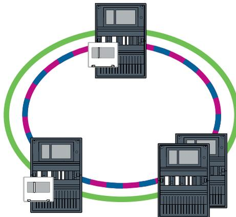
Figure 4.3: Double loop of Ethernet and CAN
