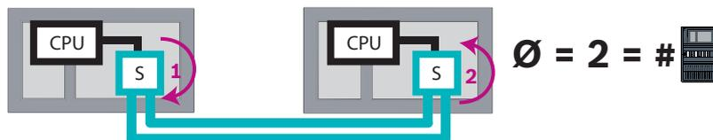
**Figure 5.1:** Network diameter of a loop with 2 panels
