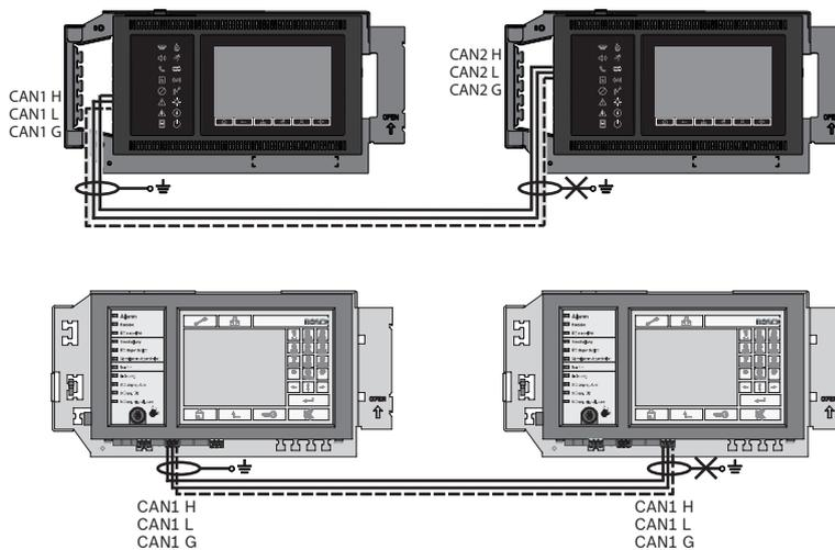
**Figure 6.1:** CAN connection (top: AVENAR, bottom: FPA)
