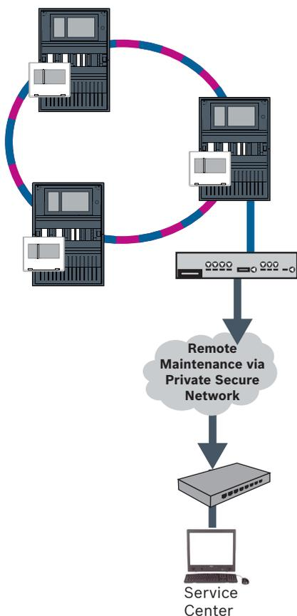
**Figure 8.5:** Remote Maintenance for Private Secure Network
