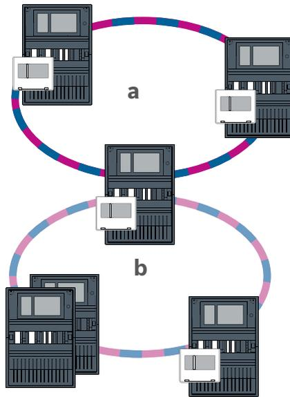
**Figure 4.6:** Connecting Ethernet loops via a non-redundant panel
