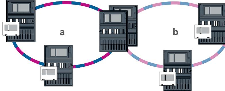
**Figure 4.7:** Connection Ethernet loops via a redundant panel
