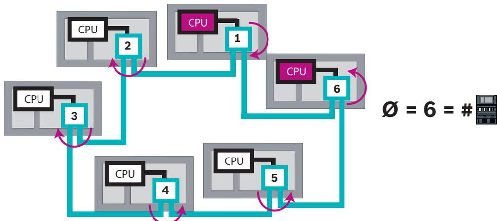
**Figure 5.2:** Network diameter of a loop with 6 panels
