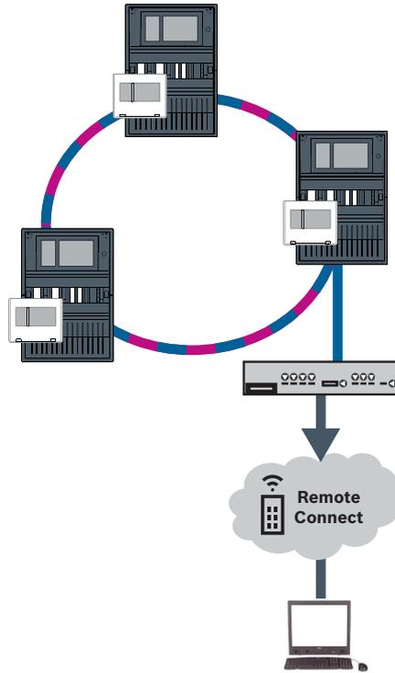
**Figure 8.1:** Remote Connect in an Ethernet loop
