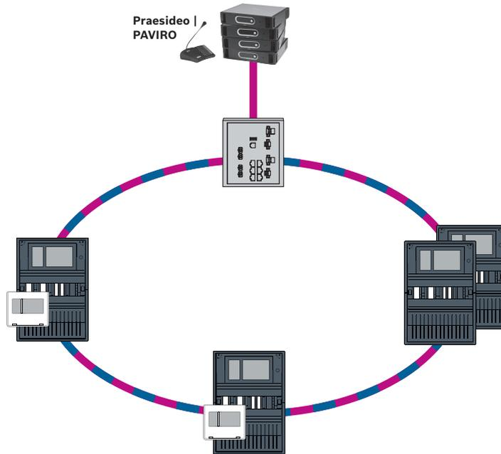
**Figure 10.4:** VAS integrated in Ethernet panel network
