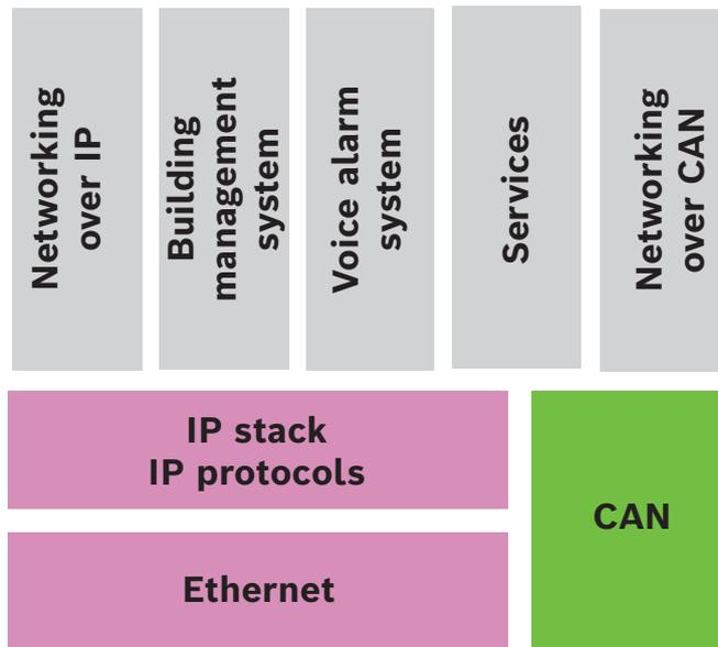
In the network, the Ethernet interface and IP protocols are used for different services. The Ethernet interface can be disabled completely or its use disabled only for networking over TCP/IP. Disabling may be necessary for networking over CAN.
