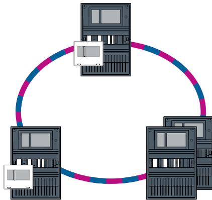
Figure 4.2: Ethernet loop
