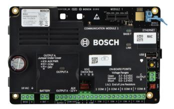
The B5512 Control Panel integrates intrusion and residential fire, providing one simple user interface for both systems. The B5512 provides up to 48 individually identified points that can be split into 4 areas.
