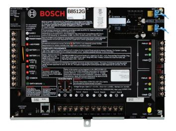
The B9512G Control Panel and the B8512G Control Panel are the new premier commercial control panels from Bosch. B8512G control panels integrate intrusion, fire, and access control providing one simple user interface for all systems.
