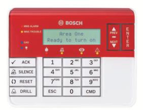
This keypad is a fully supervised SDI2 device for Mass Notification Systems and fire applications. Each keypad has user-adjustable backlit keys, a display that shows system messages, and a sounder. The sounder emits distinct condition tones to alert you to alarms, troubles, and supervisory events as they occur. The keypad includes status indicators and function keys.
