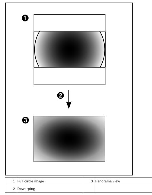
The following example figure illustrates the cropping of a 360° camera which is floor- or ceiling mounted.
