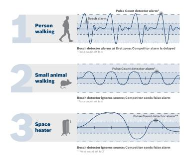
**Advanced microwave Doppler radar** – Microwave Noise Adaptive Processing uses pattern recognition circuitry to identify and ignore repetitive false alarm sources. It adjusts to background disturbances to reduce false alarms without sacrificing the ability to respond to an intruder.
