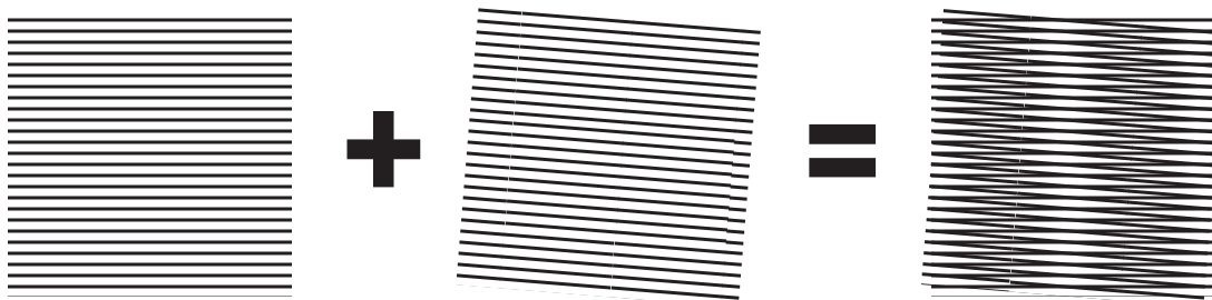
Figure 4.1: Moiré effect caused by two superimposed patterns (example)
