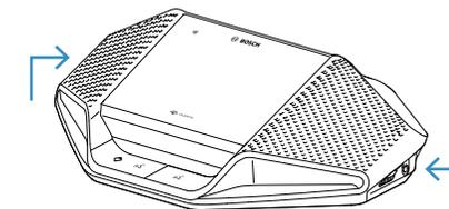
Press the triangle icon to change the headphone volume or use the volume wheel on the side of the device.
