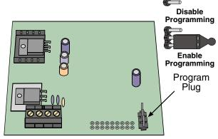
Place the Program Plug over the Enable Pins for Programming Mux Devices
