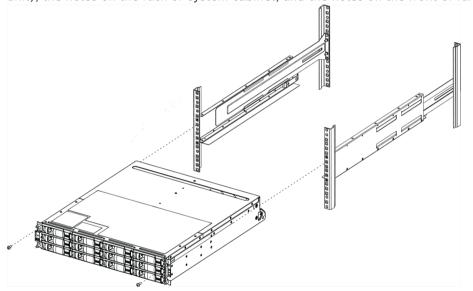
6. Secure the unit to the back of the rails by inserting two M5 screws through the brackets at the unit and the rail kit bracket.
