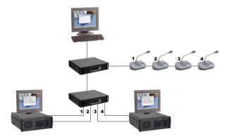
The Individual Channels software is used to route individual delegate microphone audio signals to the DCN system audio channels. These individual audio channels can only be received by Audio Expanders or Cobranet Interfaces.
