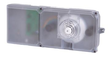
The FAD-420-HS-EN Duct detector housing with base with integrated FAD-425-O-R Detector detects smoke in ventilation ducts. Smoke particles in the air are reliably detected and reported to the fire panel by the LSN improved bus system.
