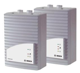
FCS-320-TP Conventional aspiration smoke detector series are active fire detection systems for early fire detection in area and equipment monitoring, as well as for the monitoring of air conditioning units or ducts (provided that the detector is installed outside of these units or ducts).
