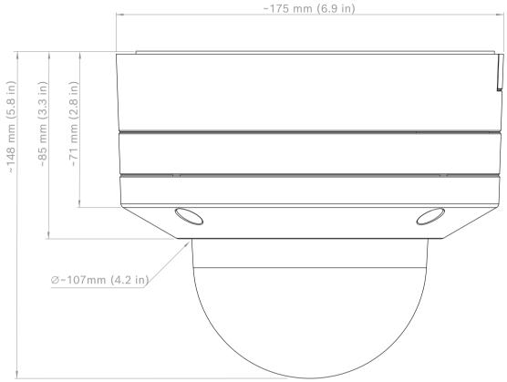
Figure 12.1: FLEXIDOME IP 8000i dimensions
