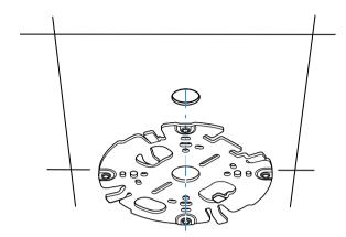
For a camera mounted on a wall: make sure that the mounting plate is oriented in a 90° angle, with the holes parallel to the floor, to allow for the use of a weather protector if necessary.
