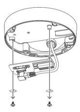
Attach the connection PCB to the camera module.
