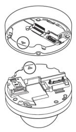
3. Remove the protective cover from the bubble.
