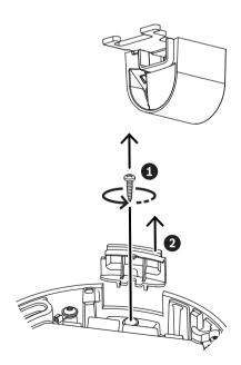
If there are auxiliary connections, puncture a hole in the rubber of the secondary cable inlet (2) in the camera base to put them through. The diameter of the whole must be between 5 and 8 mm (0.2 and 0.3 in.).
