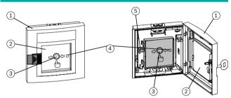
In the event of an alarm, the glass pane (2) is broken first, then the manual call point (3) is pressed hard. This activates the micro switch for alarm triggering and the indicator LED (4) blinks.
