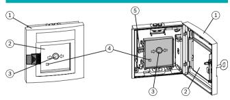
With single action call points, the alarm is triggered when the glass plate (2) is broken and the button (3) springs up.
