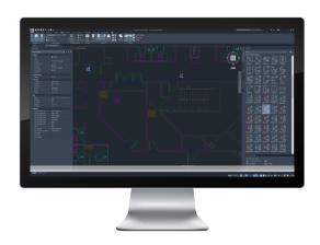
The Bosch SSD plugin supports architects, planners, specifiers, distributors and system integrators to easily and rapidly transfer the designed EN 54 fire alarm devices from AutoCAD® software to Safety Systems Designer, where the further planning steps can be handled (preparation of the bill of materials and tender text, battery calculation, check of the system viability, aso).
