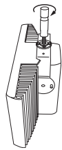
Figure 5.7: Attaching the stud of a floor stand to the suspension bracket of the radiator
