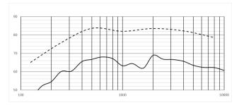
Fig. 4: Frequency response graph (-1/3<sup>rd</sup> octave dB SPL @1 W(100 Hz - 10 kHz), 4 m; - 1/1th octave dB SPL @1 W(100 Hz - 10 kHz), 1 m)
