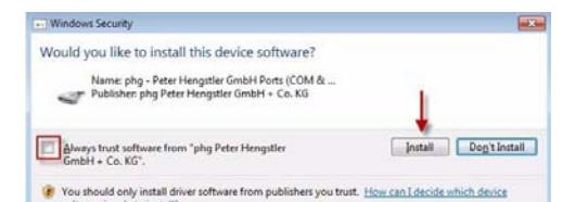
After installation is completed successfully the reader can be used under the newly installed virtual COM Port (see Windows Hardware Manager for port number).
