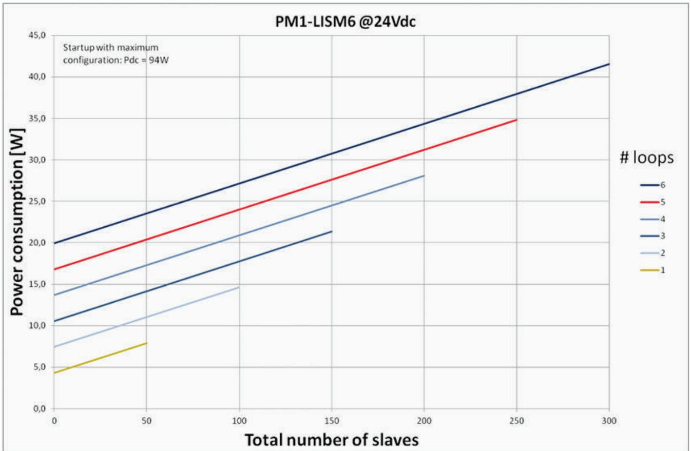
Figure 11.1: Battery power consumption 24 Vdc
