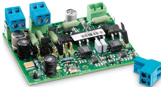
The Isolator Board has two 100 volt audio connectors for connecting to both sides of the loudspeaker loop and a third 100 volt audio connector for creating a tap-off for one or more loudspeakers. Jumper settings are provided to set the permissible loudspeaker power level (10, 36, 100 watt, or 10 watt with 20 kHz pilot tone filter), and other supervision settings.
