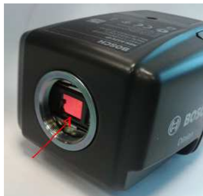
Frame of the switching IR filter Positioned at max physical boundary
