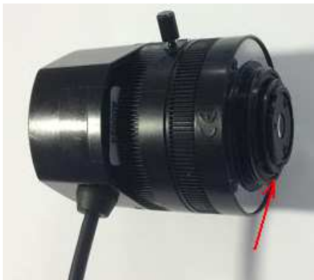
Focus far / infinity Inner tube in max position
