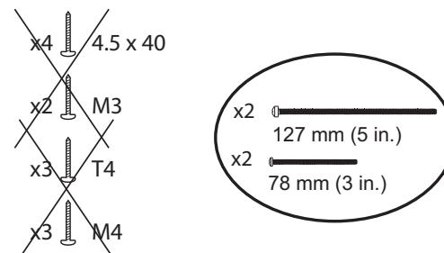
Note: When installing some FLEXIDOME cameras (such as NIN-70122-FOA), use the M4 washers to prevent the screw head from falling through the mounting hole.
