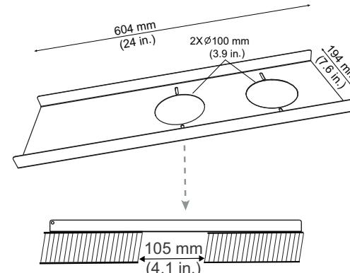
Note: FLEXIDOME IP panoramic 7000 MP cameras require a mounting plate between the camera and the ceiling, as illustrated in item a in the following figure. Other FLEXIDOME cameras can be mounted directly to the ceiling.
