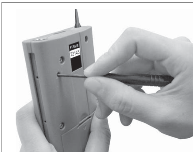
figure 5.4: Adjusting the sensitivity
