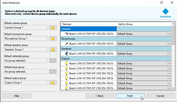
8. This is how the IP horn/amp should appear in the VMS (1 Camera, 1 Microphone (only for the IP horn), 1 Speaker, 33 Outputs).
