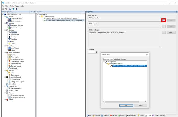
3. To assign a loudspeaker to the camera click on the three dots next to *Related speaker*. A Popup window will open, and you need to select the speaker of the IP horn/amp and click *OK*.
