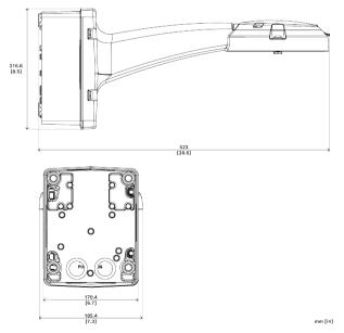
These units can be mounted directly to a wall or other flat surface. Optional pole and corner mounting accessories are also available, allowing you to tailor your AUTODOME installation to your specific requirements. Multiple cable gland/conduit entry points protect cables and simplify installation.
