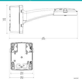
These units can be mounted directly to a wall or other flat surface. Optional pole and corner mounting accessories are also available, allowing you to tailor your AUTODOME installation to your specific requirements. Multiple cable gland/conduit entry points protect cables and simplify installation.
