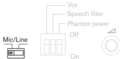
Figure 6.3: VOX input source switch
