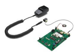
The basic call station kit is an open frame call station to create dedicated full custom operator panels for PRAESENSA Public Address and Voice Alarm systems. It has the same functionality as the PRA-CSLW, but without LCD user interface to facilitate easier mounting in operator desks or in wall-mounted fireman's panel enclosures. It comes with a detachable, supervised omnidirectional fist microphone for close talking with press-to-talk button and a separate small monitor loudspeaker.
