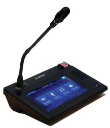
The PRP-CST is a desktop call station with a touch screen and gooseneck microphone, capable of connecting to the PROSPERO Public Address System via a standard IP network for manual and prerecorded announcements. The call station supports PoE, allowing connection to a standard Ethernet switch using a Cat5e cable.
