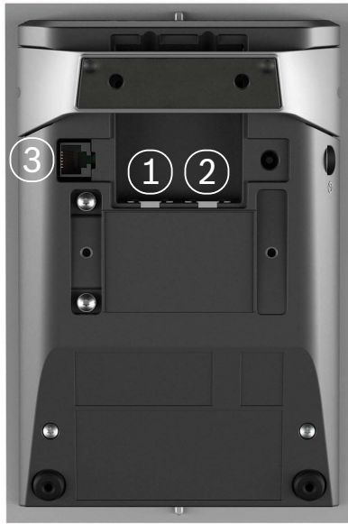
Figure 3.13: Rear view of PRA-CSLW: Network port (1-2) connection. Interconnection to PRA-CSE (3)
