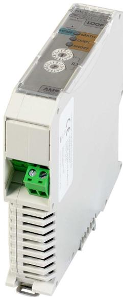
LDB (LoopDrive Booster), with ordering number PRA-LID - is the central unit installed in the Voice Alarm System rack, directly between the amplifier and loudspeaker line. Mounted on a DIN-rail LDB works as the DC-power supply for FIMs and can also generate special service commands to FIMs.
