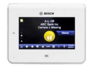
**Camera missing:** The intrusion system has lost supervision with IP camera #1 (e.g. camera is damaged)
