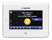
**Camera tamper:** The intrusion system is supervising an IP camera with a camera tamper condition (e.g. camera has been obstructed).
